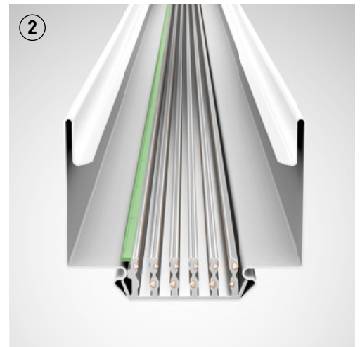
11-core current conducting profile 5 \times 2.5 \text{ mm}^2 + 6 \times 1.5 \text{ mm}^2 3 separate circuits 2 control lines for DALI signal 2 independent emergency light circuits
